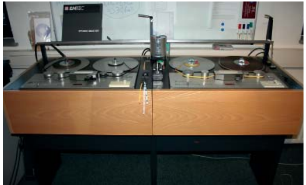
Telefunken AEG M20 as feed to twin console with two Telefunken M15a as copy station
