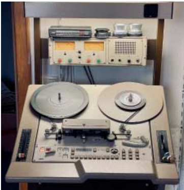
Telefunken AEG M20 as feed to twin console with two Telefunken M15a as copy station
